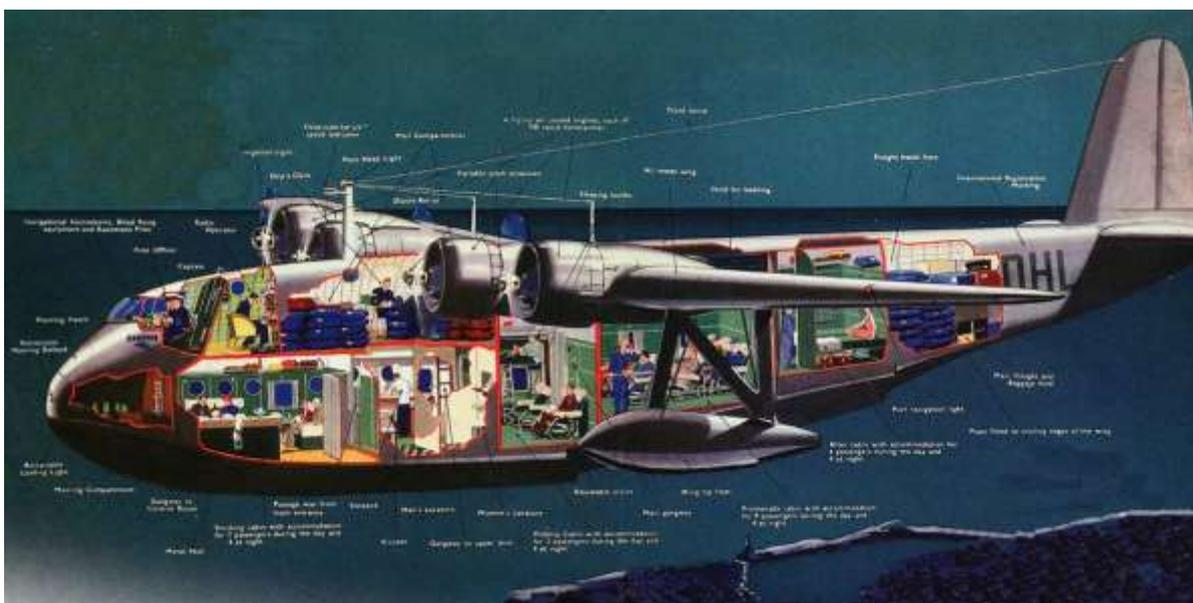
*Cutaway view of an S.23 Empire boat. Clearly shown is the double deck layout with the Flight Clerk (later redesignated as Purser), located at the rear of the flight deck. Due to larger than anticipated volumes of EAMS mail and freight being uplifted, his station was repositioned in the forward passenger cabin.*
