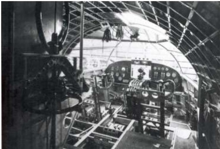
*The "Control Deck" as referred to by Shorts, was a spacious area for the technical crew to work in. Rudder, elevator trim and flap operating switch were located above the windscreen between the two pilots. The four engine starter switches were mounted above the central coaming. Just visible at left, is the Direction Finding (D/F) loop antenna which required pushing up into the airstream.*
