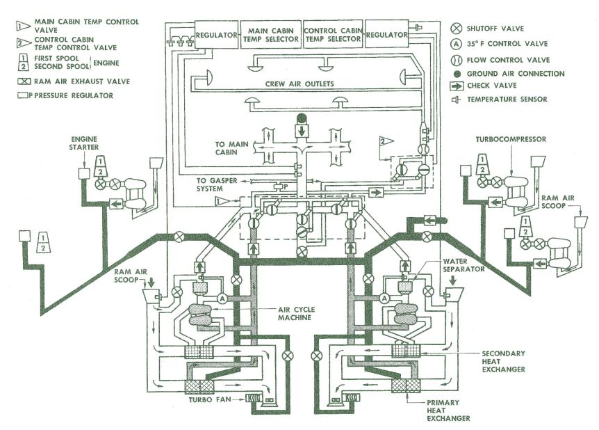
AIR CYCLE AIR CONDITIONING SYSTEM SCHEMATIC
