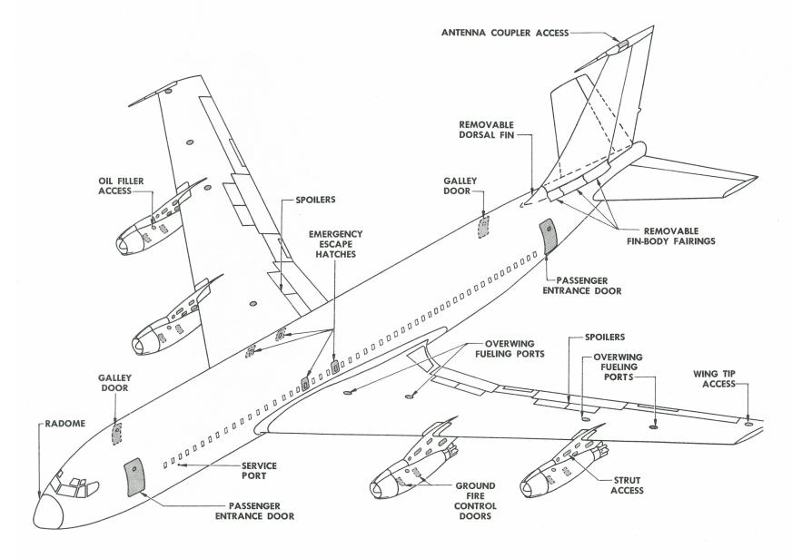
ACCESS DOORS AND INSPECTION OPENINGS—TOP VIEW
