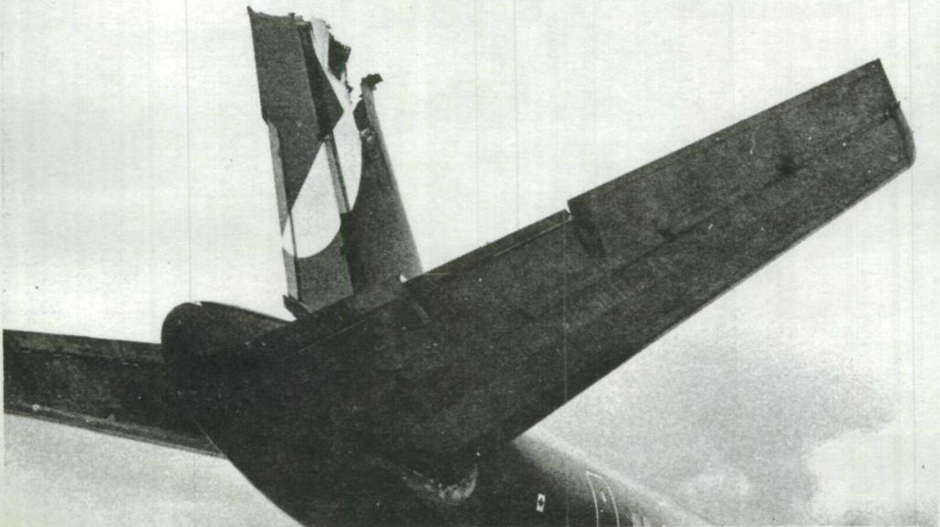
FIG. 4 Damage sustained by tail fin and rudder of CF-CPQ.
