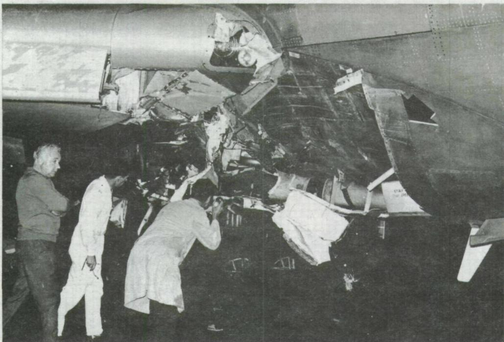
FIG. 1 Damage to VH-TJA in forward wing root area on starboard side. The arrow indicates the point of first contact.
