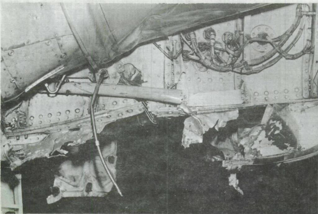
FIG. 2 View from within starboard wheel bay of VH-TJA, showing damage sustained by forward bulkhead.
