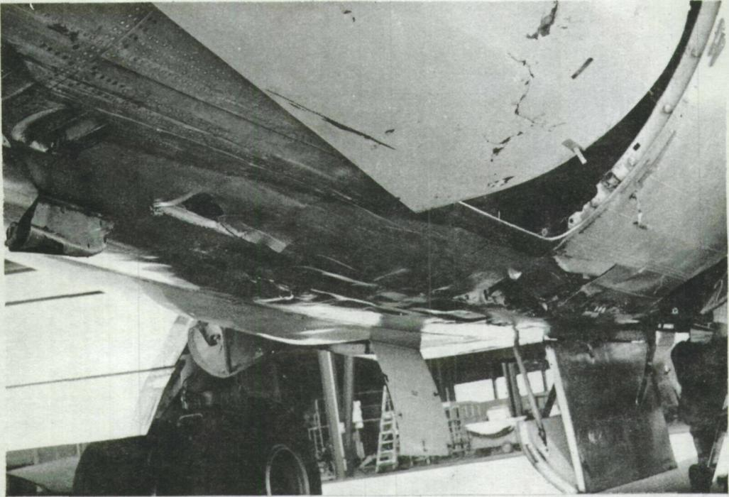
FIG. 3 Underside of fuselage of VH-TJA showing score marks and punctures between starboard wheel bay area and tail bumper.
